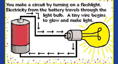
If the flow of electrons is broken at any place on the circuit the appliance will stop working. For exam-
